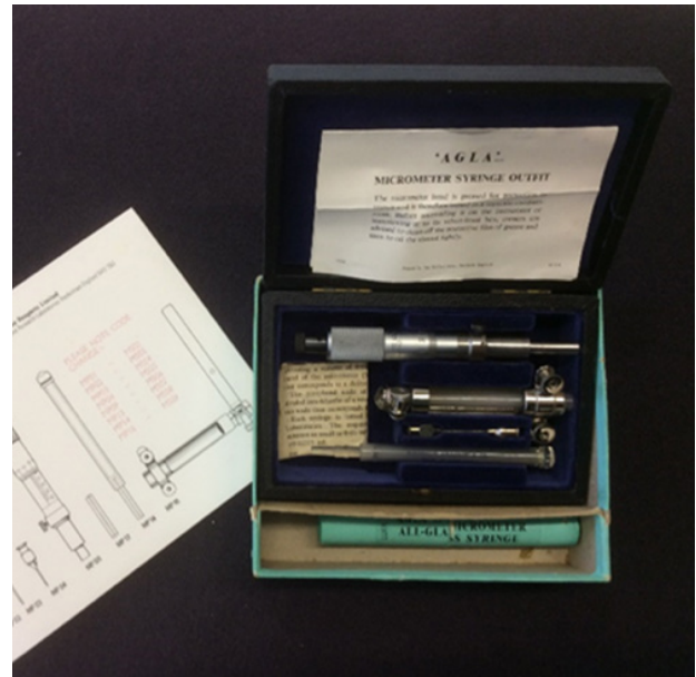
Fig. II: A micrometer-controlled syringe for accurate small amounts possibly for research or clinical use in toxicology and immunology
